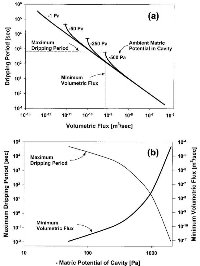
**Figure 6.** Theoretical dripping characteristics determined by decoupled (independent) liquid flux and evaporative conditions (matric potential of cavity) for a groove angle  $\gamma = 30^\circ$ . (a) Dripping period under different cavity ventilation conditions (matric potentials) dependent on volumetric flux. (b) Minimum volumetric flux required to generate dripping under different ventilation conditions (matric potential of cavity) and the associated maximum dripping period.
