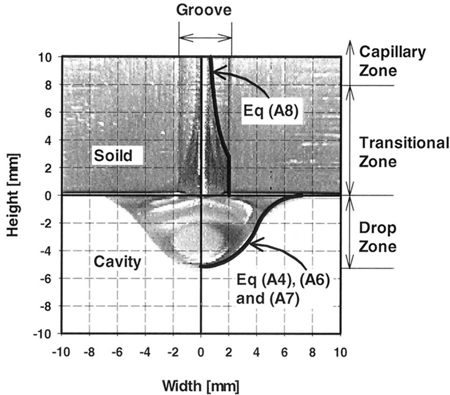
**Figure A1.** Classification of the dripping flow regime into capillary, transitional, and drop zones. Solid outlines are theoretical profiles of transitional and drop profiles calculated according to simplified methods discussed in appendix A (fixed variables are  $L = 3.5$  mm,  $\gamma = 60^\circ$ ,  $\theta = 0^\circ$ ,  $\lambda = 1.3$ ; solved variables are  $\phi = 0.02$ ,  $\alpha = 0.75$ ,  $a = 4.5$  mm, and  $R = 5.7$  mm).
