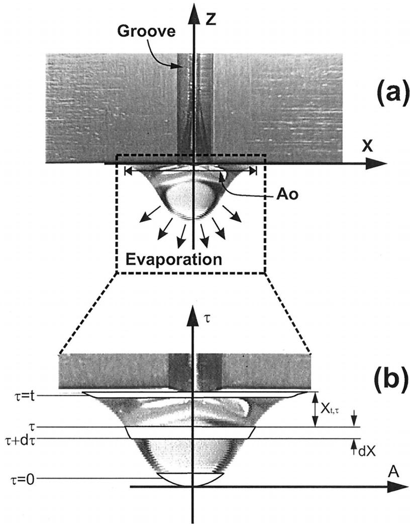
**Figure 2.** Definition diagram showing a drop forming into a cavity from the face of a fracture roughness model (aluminum slab with vertical grooves): (a) Cartesian coordinate system and (b) Lagrangian coordinate system. Elements of the drop in horizontal plane are marked by a moving (in time).
