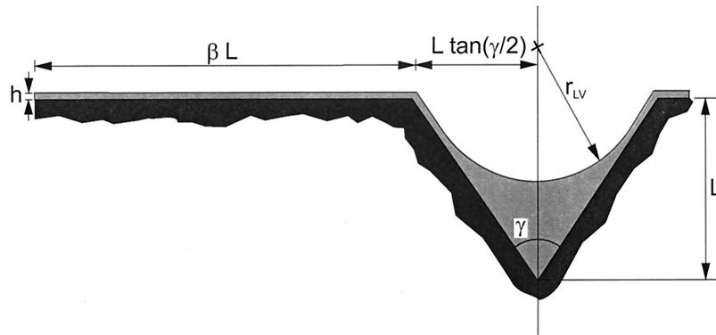
**Figure 1.** Definition sketch of a unit fracture surface-roughness element in a horizontal cross section. A groove is defined by its depth ( $L$ ) and angle ( $\gamma$ ). The attached plane for film flow is proportional to the groove depth with coefficient  $\beta$ .
