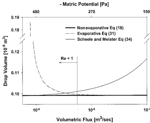
**Figure 5.** Comparison of drop volume under nonevaporative (equation (18)) and evaporative conditions (equation (31)) with a semiempirical equation of *Scheele and Meister* [1968] (equation (34)).
