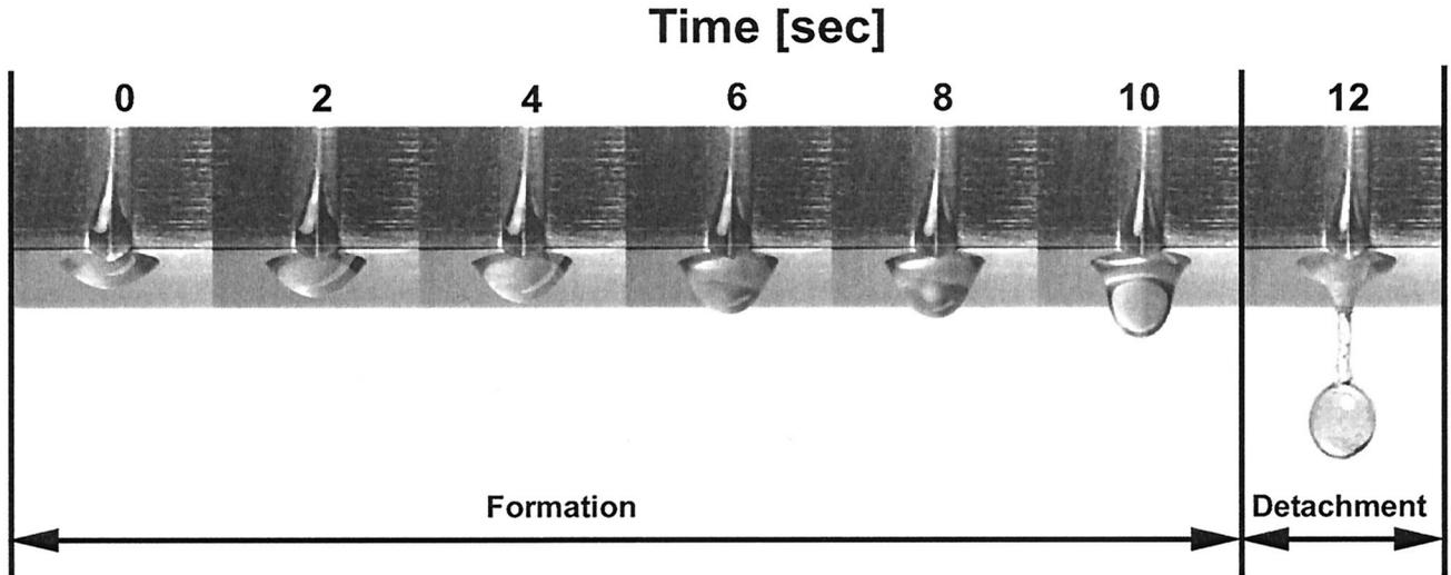
**Figure 3.** Time sequence photographs of water drop formation and detachment from vertical grooves ( $L = 3.5$  mm,  $\gamma = 60^\circ$ , and  $Q \cong 1$  cm<sup>3</sup> min<sup>-1</sup>). Note that the drop anchoring area ( $A_o$ ) does not change. The drop has approximately hemispherical shape for the first 5/6 time of the total formation period (drop formation period); in the remaining 1/6 of the period the drop forms a neck and detaches (drop detachment period).
