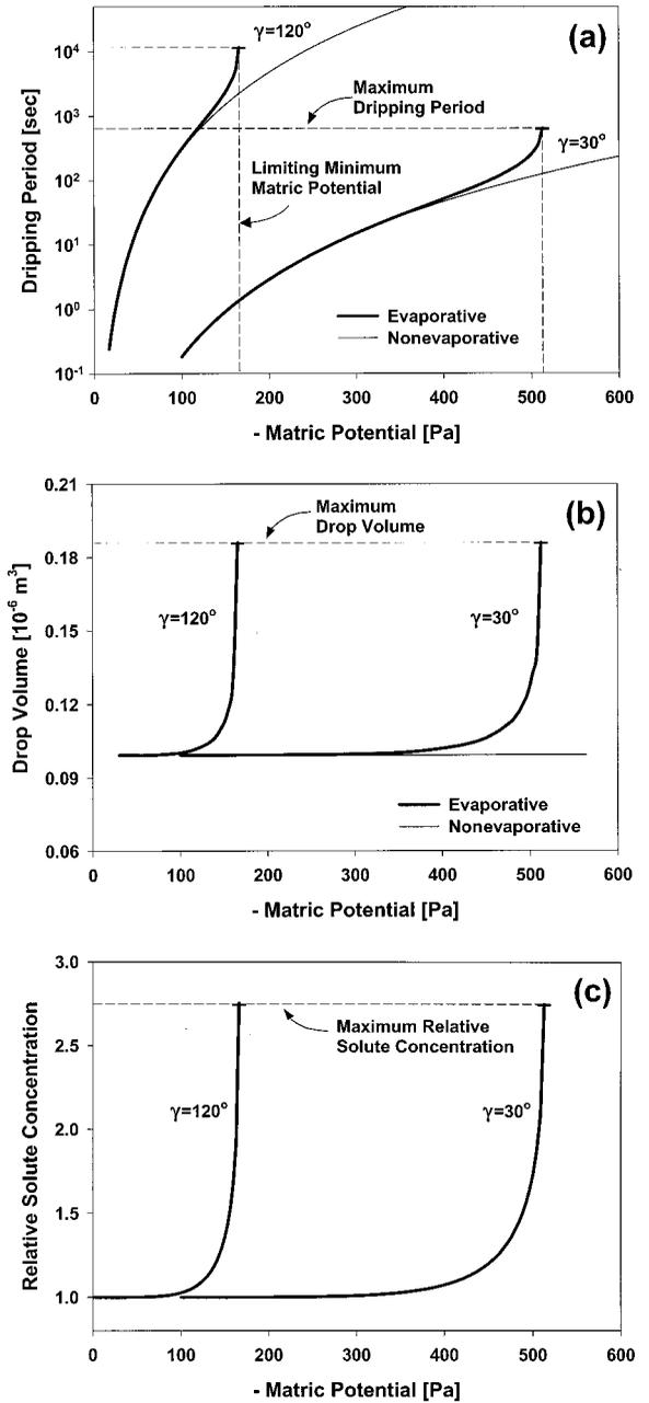
**Figure 4.** Theoretical dripping characteristics dependent on coupled matric potentials ( $\psi$ ) of cavities and fractures. (a) Drop detachment time ( $\tau_c$ ) under evaporative and nonevaporative conditions. (b) Drop volume at detachment under evaporative and nonevaporative conditions. (c) Relative solute concentration of drops at detachment time.
