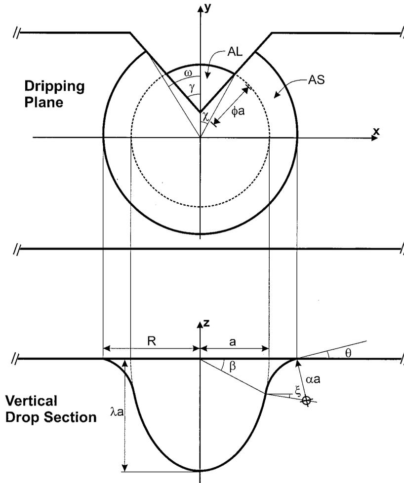
**Figure A2.** Schematic diagram of the simplified drop model used to calculate drop anchoring area and drop profile.
