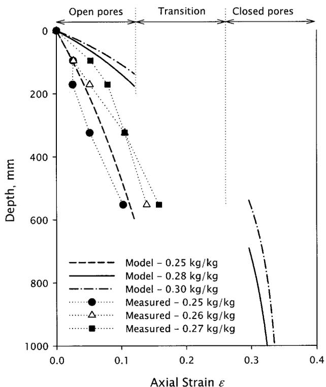
Fig. 7. Strain profile in Millville silt loam soil. Measured values correspond to soil columns of soil passing through 2-mm sieve (Ghavami et al., 1974). Model values correspond to calculations using an aggregate bed made of 2-mm aggregates.
