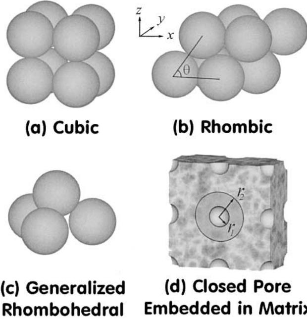
Fig. 1. Basic structural units. (a) Spheres in cubic packing, (b) spheres in rhombic packing, (c) generalized rhombohedral unit, and (d) spherical pore of radius  $r_1$  embedded in homogeneous spherical matrix of radius  $r_2$  ( $r_1 - r_2$  is the thickness of the solid shell associated with the given pore).
