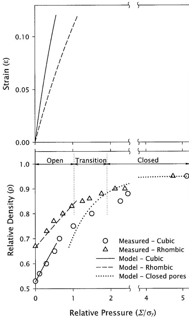
Fig. 5. Coalescence of modeling clay under isotropic stress. (a) Strain as a function of dimensionless stress. (b) Relative density as a function of dimensionless stress, for two packing angles. Note that for closed pores the original packing is irrelevant.
