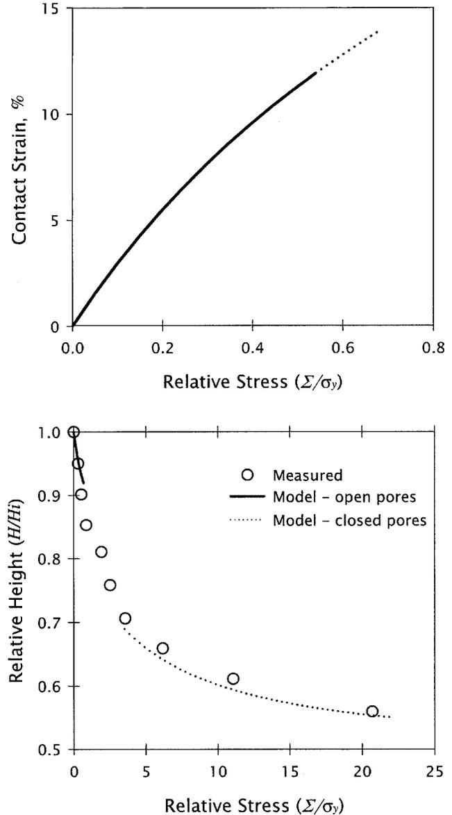
Fig. 6. Coalescence of natural soil aggregates under uniaxial stress, at constant strain rate. (a) Strain as a function of dimensionless stress. (b) Relative density as a function of dimensionless stress.
