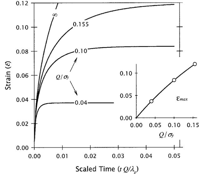
**Fig. 3. Viscoplastic strain of a generalized rhombohedral system as a function of nondimensional time for various dimensionless load ratios. Inset: The maximum strain as a function of the dimensionless load ratio (circles denote the load-ratio values used in the main plot).**
