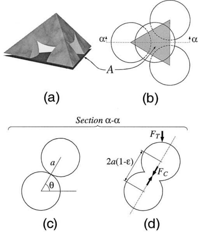
Fig. 2. Definition of variables for the generalized rhombohedral system. (a) Truncated unit cell, (b) planar area of the unit cell, (c) packing angle, and (d) strain.
