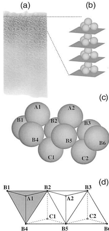
Fig. 4. Conceptual model of soil aggregate bed. (a) Schematic representation of soil aggregate bed, (b) one-dimensional array of unit cells separated by conceptual rigid planes (c) one layer of close-fitting unit cells, (d) planar view of a layer of unit cells.
