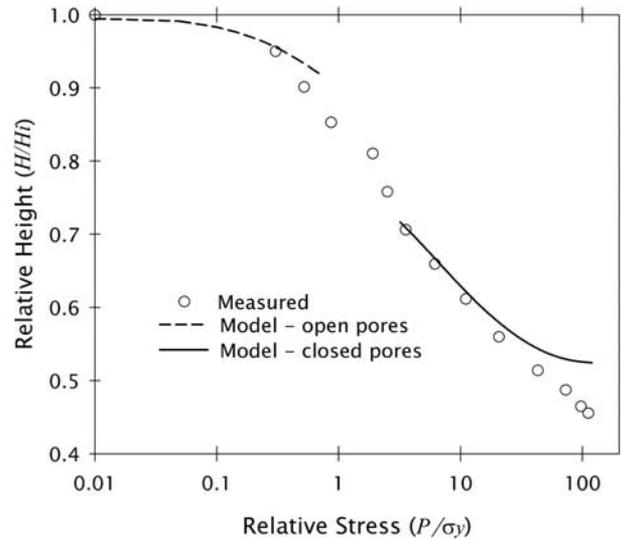
**Figure 6.** Densification of natural soil aggregates under uniaxial stress at constant strain rate, expressed in terms of relative density as a function of dimensionless stress.
