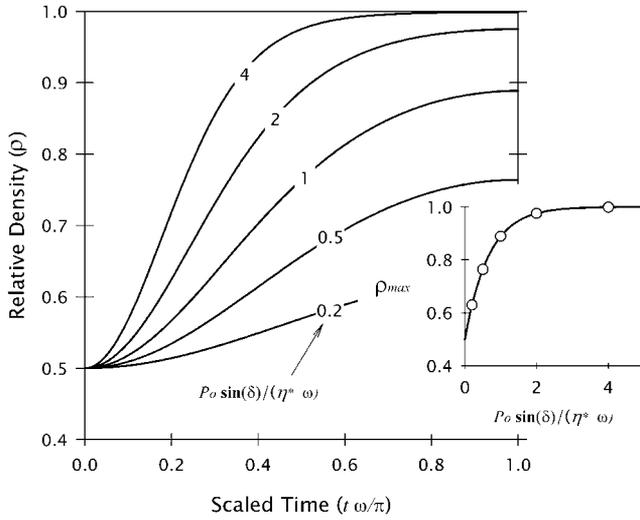
**Figure 4.** Viscous component of densification resulting from transient stress as a function of nondimensional time for various dimensionless load ratios. Inset shows the maximum strain as a function of the dimensionless load ratio (circles denote the load-ratio values used in the main plot).
