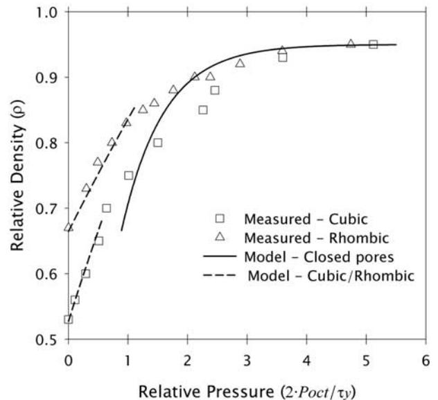
**Figure 5.** Densification of oil-based modeling clay under isotropic stress for two packing angles, expressed in terms of relative density as a function of dimensionless stress.
