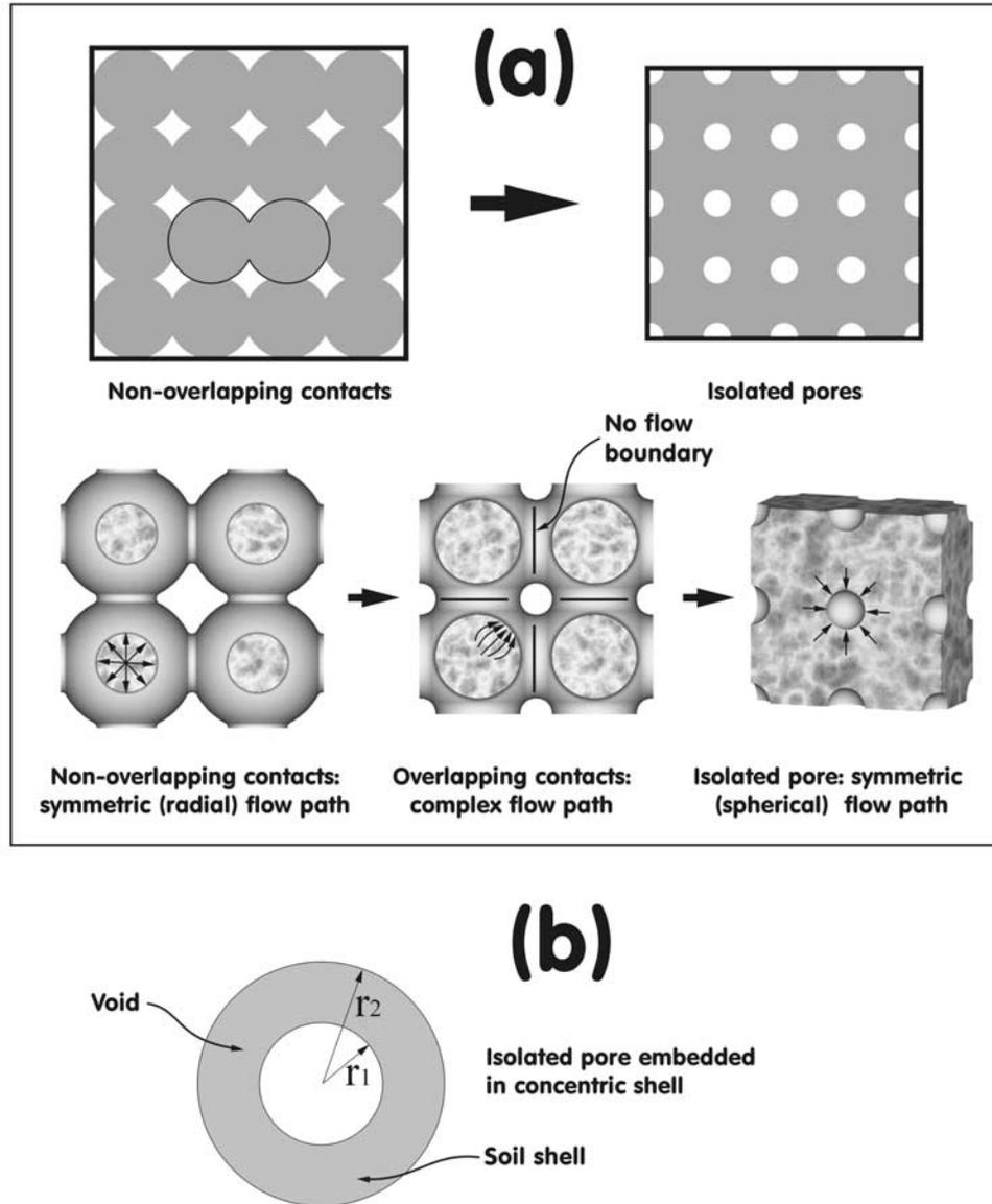
**Figure 2.** (a) Schematic representation of the transition from open pores to closed pores. Note that for the open pores and closed pores the flow paths are symmetrical, whereas the transition has an asymmetrical complex flow path. (b) Definition of closed pore.
