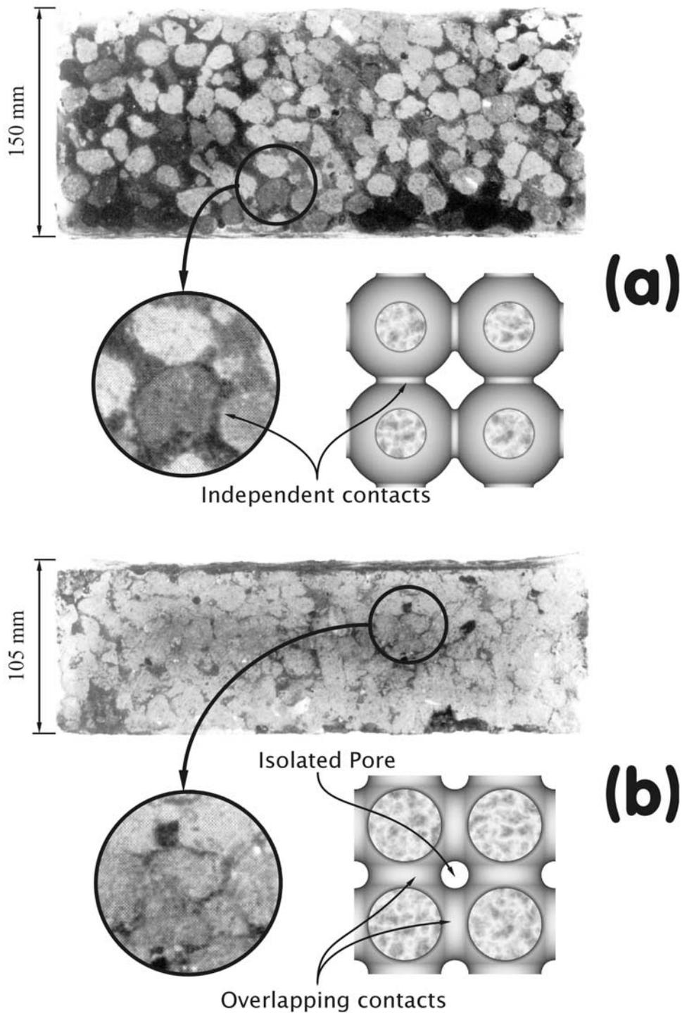
**Figure 1.** Transition from open pore geometry to closed pore geometry in aggregated soil subjected to axial stress [Braunack et al., 1979]. After the aggregates have been deformed, adjacent interaggregate contacts begin to touch each other. The analogs using the conceptual model of this study are shown.
