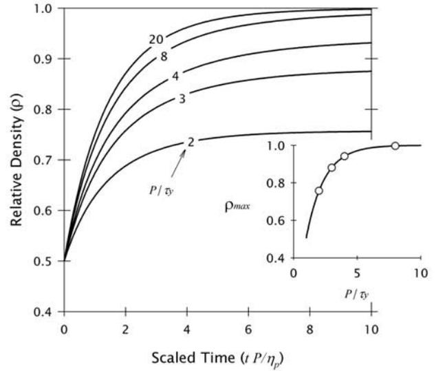
**Figure 3.** Viscoplastic densification of isolated pore as a function of nondimensional time for various dimensionless load ratios. Inset shows the maximum strain as a function of the dimensionless load ratio (circles denote the load-ratio values used in the main plot).
